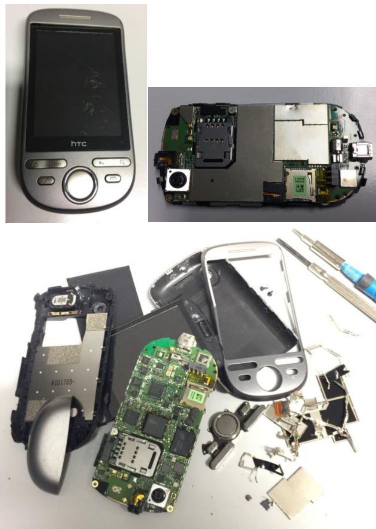
Figure 13. Photographs illustrating the procedure of dismantling a mobile phone. Top left: intact mobile phone, top right: circuit board of the mobile phone with metal sheets covering the components, bottom: all parts of the mobile phone after dismantling.
