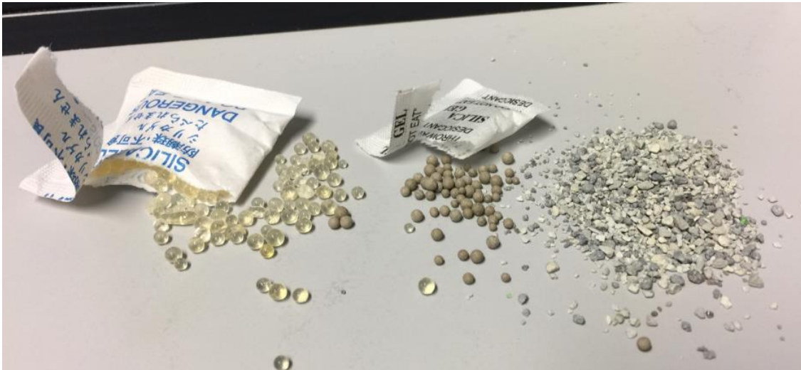
Figure 9. Different types of desiccants. “Silica gel” bags found in hand bags (left and middle) and cat litter (right).
