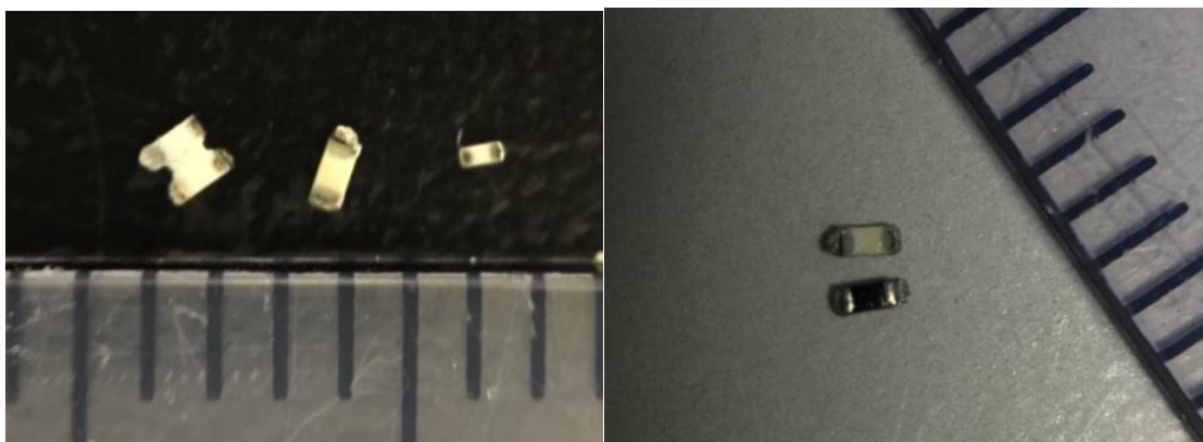
Figure 14. Different sizes (left) and the black upper side and white underside of the SMRs with dosimetric properties. Each gradation on the scale denotes one millimetre.
