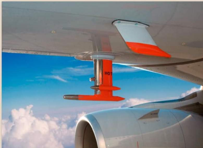
Detail from the wing of a Lufthansa Airbus 340-600 used in the IAGOS-CARIBIC project, showing the inlet for air and aerosol particles for atmospheric aerosol sampling.
