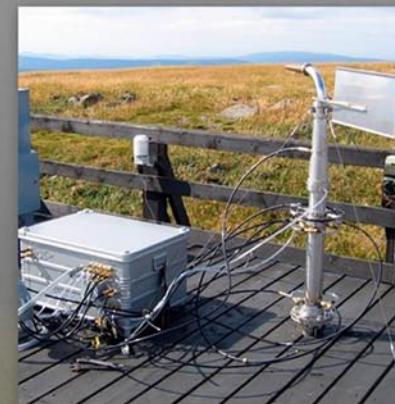
Cloud studies using the droplet aerosol analyser (DAA) on Mt Brocken in Germany, 2010. The DAA set up for field measurements.
