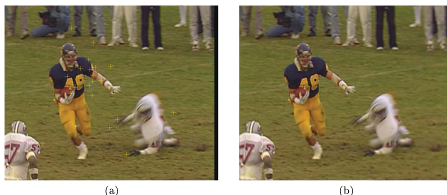
Fig. 1. Example of offline foveation. The left picture shows where people look in the original frame and the right picture depicts the same frame after offline foveation. Each crosshair represents one viewer's position of gaze. Peripheral blurring due to offline foveation enables more efficient compression.
