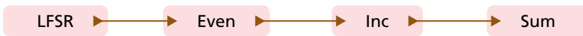
Figure E.9: A program with four processes. LFSR is a linear feedback shift register, producing the n = 10^7 first numbers of a maximum length sequence of 16 bits, followed by a 0. Even filters out all odd values, forwarding only the even numbers to Inc , that increments the numbers by 1. Sum computes the sum of all numbers until it gets a 1 (the incremented 0 at the end of the stream) and prints the sum.
