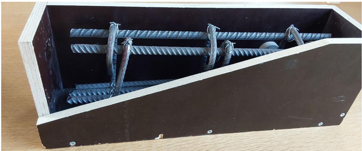
Figure C.2. Concrete reinforcement and formwork (cut for demonstration purposes)
