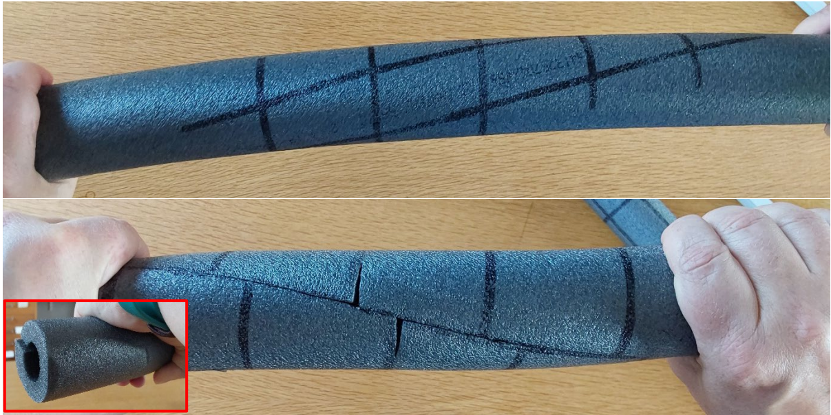
Figure C.4. Foam pipe insulation (top) without and (bottom) with slit to demonstrate warping of open cross sections
