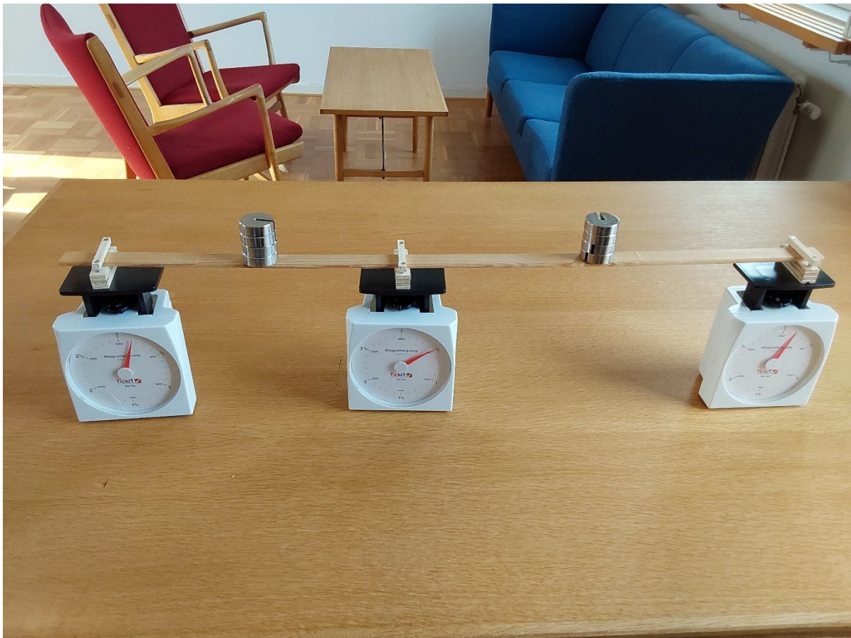
Figure C.12. Bending of a thin timber beam element with variable position of supports and loads. The scale also provide the reaction forces.
