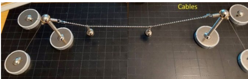
Figure C.3. A hanging cable showing funicular form for varying load placements (using Mola® kit)
