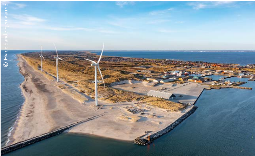
FIGURE 1: The wind turbines at Hvide Sande, Denmark. Effect: 3 x 3 MW. Height: 140 meters.
