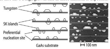
**Figure 1** Preferential nucleation of Stranski-Krastanow islands along tungsten lines at 600°C and V/III = 14
