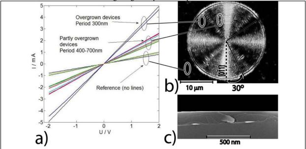
**Figure 4 a)** IV characteristics of measured devices. **b)** SEM image of overgrown tungsten circles and **c)** cross-section of overgrown InAs over W-grating aligned 30° off from the [011]-direction.
