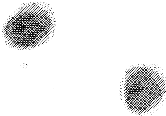
Figure 1.13: The first proton nuclear magnetic resonance zeugmatogram, i.e. MRI picture by Lauterbur [128], depicting a transversal slice through two test tubes containing water. Reproduced with permission from Nature Publishing Group.
