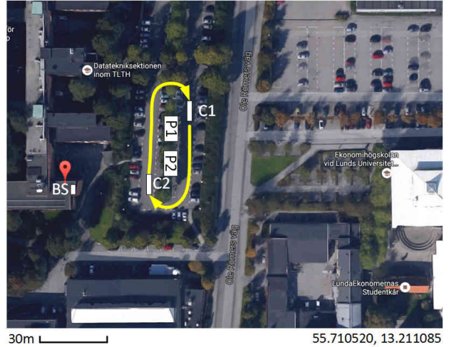
Fig. 3. Overview of the measurement scenario at the campus of the Faculty of Engineering (LTH), Lund University, Sweden. Arrows indicate the direction of movement for the cars C1 and C2. Pedestrians P1 and P2 moved within the zones indicated by their white boxes.
