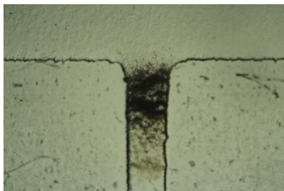
Figure 3.4: Aluminium salts forming gel plugs within PDMS devices, viewed with optical microscopy by BGG in preparation work for the microfluidic SAXS experiments carried out within this thesis. For scale, the vertical channel has a width of 300 \mu\text{m}
