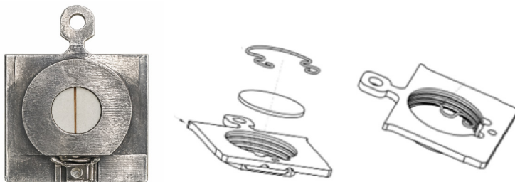
Figure 3.9: PEEM sample holder and assembly. Photograph of a PEEM sample holder together with schematic illustrations of its assembly. The sample is mounted in the central aperture and secured using a clip and back plate, ensuring good electrical contact and proper alignment for PEEM measurements.
