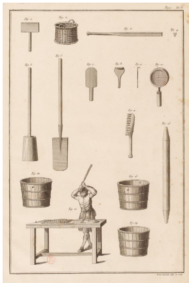
Figure 28. Depiction of the tools used during processing of the clay and the beating of the clay from Duhamel du Monceau (1771).
