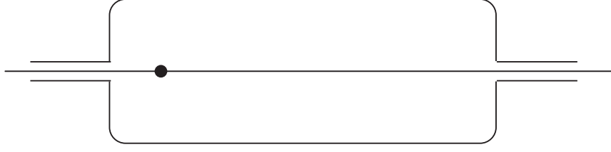
Figure 7.5: The metallic sphere on the symmetry axis of an axially symmetric cavity. The frequency shift of the mode number n is proportional to the square of the electric field at the position of the sphere of the same mode.
