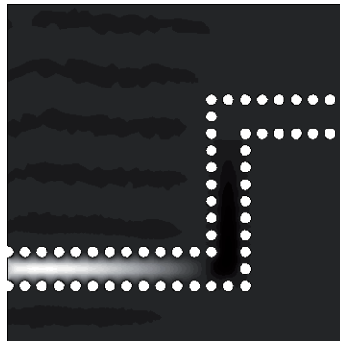
Figure 6.27: A COMSOL simulation of the SIW at 30 GHz. No modes are propagating since the frequency is below the cut-off frequency for the fundamental mode.
