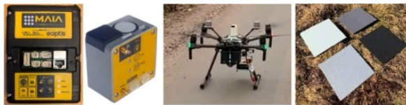
Figure 1: From left to right: The MAIA camera used to collect VNIR images, the MAIA ILS, the DJI Matrice 210 RTK drone, and the radiometric reference targets. Images from [11]
