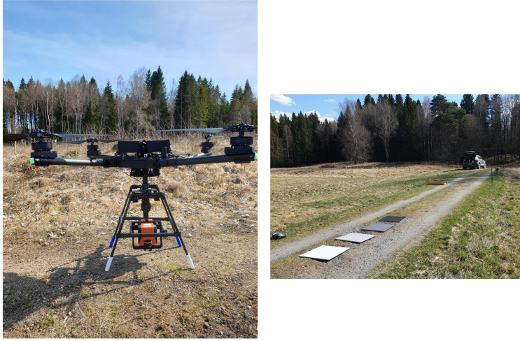
Figure 4.4: From left to right: The Freefly Alta X drone with the SPECIM AFX17 hyperspectral sensor used for data acquisition, and ground calibration targets used for post-processing reflectance estimation [14].
