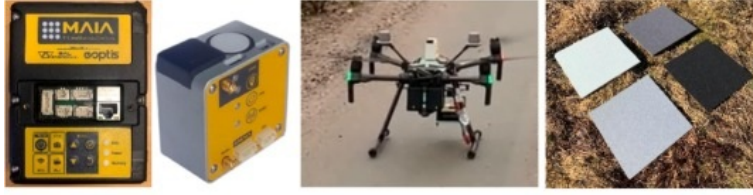
Figure 4.3: From left to right: The MAIA camera, the MAIA ILS, the DJI Matrice 210 RTK UAV, and the radiometric reference targets. Images from [40]
