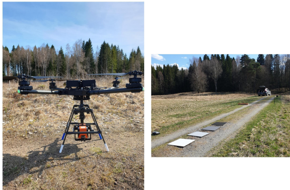
Figure 2: From left to right: The hyperspectral drone system used for acquisition of SWIR data. Ground calibration targets used for post-processing reflectance estimation. Images from [5].
