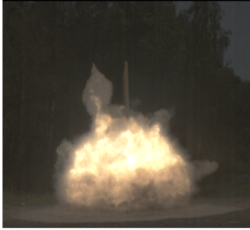
Figure 8.2: Snapshot of a video from a TNT/Al HoB 0.5 m case at \sim 3 ms.
