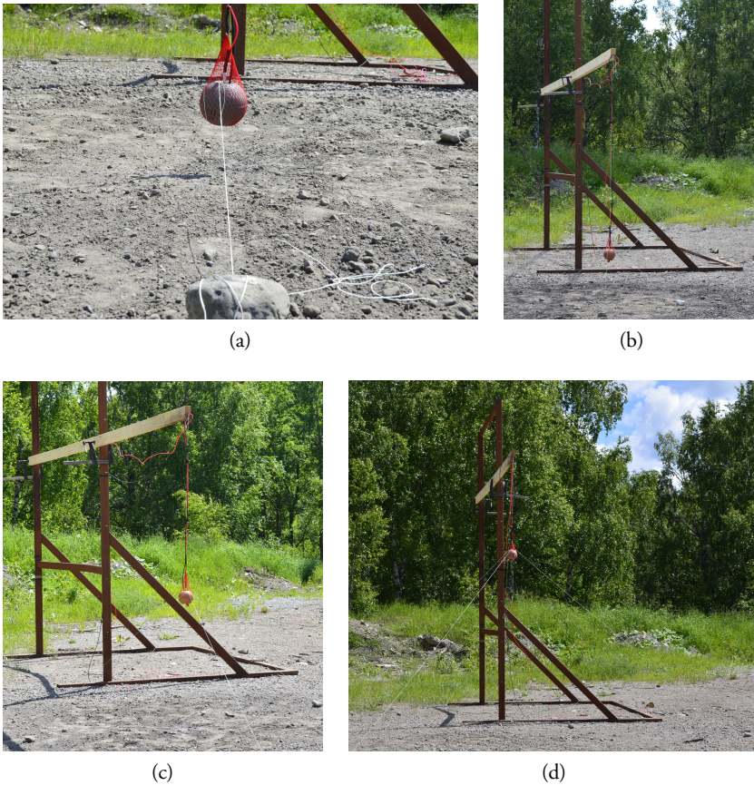
Figure 6.4: Four HoB varied in the experiments (a) 0.15 m, (b) 0.5 m, (c) 1.0 m and (d) 2.0 m.
