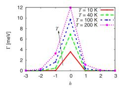
FIG. 6. (Color online) Scattering strength due to impurity layers in neighboring periods with index h. At low temperatures, screening is efficient and scattering is spatially local. When the temperature is increased, scattering at the impurities in the same period is increased, and scattering at impurities in neighboring periods becomes important.
