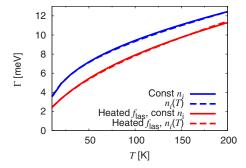
FIG. 3. (Color online) Scattering strength calculated by RPA-3 for different choices of band temperatures and densities. The temperature dependence of subband populations  $n_i(T)$  hardly changes the results, while increasing the temperature of the lasing subbands by 100 K lowers the scattering strength.
