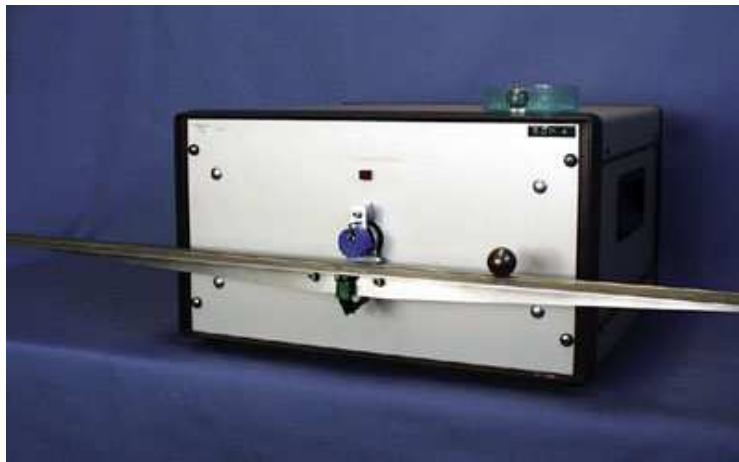
Figure 14: The ball and beam process used in the control experiments.
