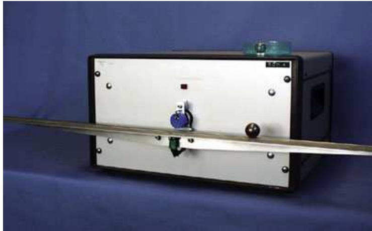
Figure 14: The ball and beam process used in the control experiments.
