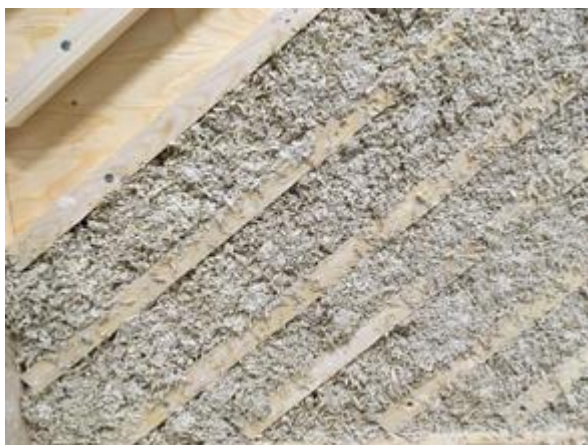
Figure 6. Testing workability of lime-hemp in between wooden slats in the lab.
