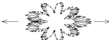
Figure 4: For stretching in the x -direction (displacement d_1 ), we plot the traction vector along the inclusion/filler interface.
