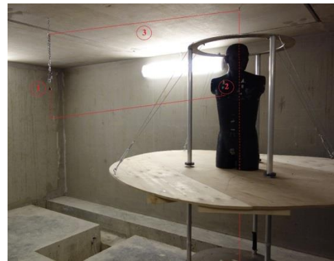
Fig. 3. Experimental setup during irradiation. 1: ^{60}\text{Co} -source mounted on a chain; 2: distance between ^{60}\text{Co} -source and personal dosimeter (1.5 m); 3: distance between ^{60}\text{Co} -source and the center of rotation.
