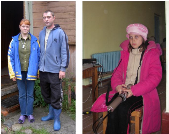
Fig. 1. Measurements in Russia. To the left: participants wearing TLDs in a cord around the neck. To the right: measurement of the ^{137}\text{Cs} body burden using NaI(Tl) detectors in a sitting position.
