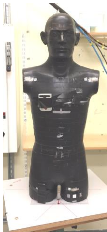
Fig. 1. The Alderson RANDO Phantom positioned on a rotating table for allowing exposure in AP-, PA- and ROT 60 Co-exposure geometries. TLDs and an EPD were positioned on the phantom in chest height. A portion bag with salt was put at the height of the trouser pocket on the front side of the leg.
