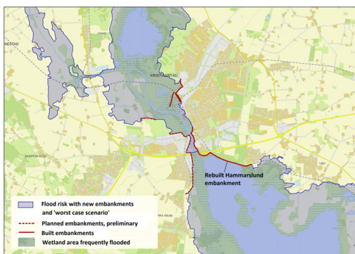
Fig. 7. Flood risk with new embankments and 'worst case scenario'. The wetland areas with different degree of wetness including flooded meadows are continuing to function as buffer zones.
