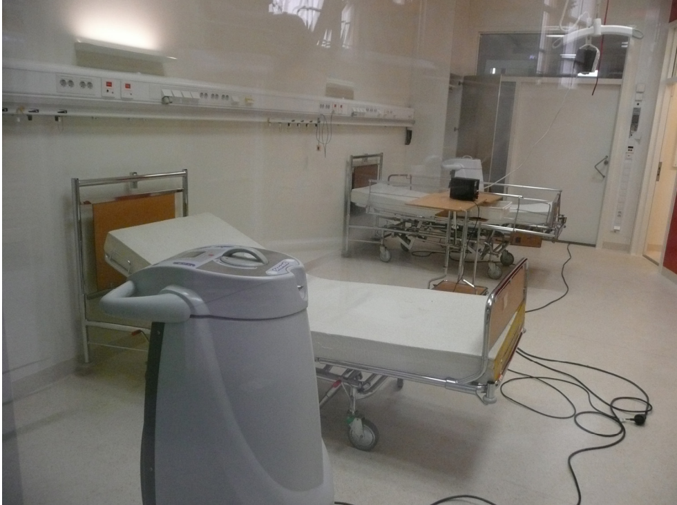
Figur 9. Two aHP devices (Run by Bakterifritt) in action in the mock up during study 2. Photo Torsten Holmdahl
