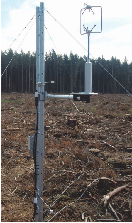
Figure 5. One of the three m tall masts equipped for flux-gradient measurements of CO 2 , CH 4 and N 2 O. The sonic anemometer was mounted at 2.5 m height and the air intakes were at 0.6 m and 2.0 m but were adjusted for increasing height of the vegetation. Photo by Patrik Vestin.
