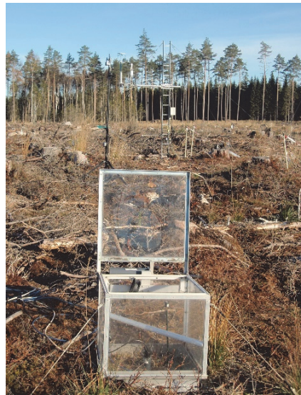
Figure 3. One of the automatic chambers used for measurements of CO 2 and CH 4 fluxes from the forest floor (Papers I and III). Here, measurements of CH 4 exchange at a clear-cut and soil scarified plot in 2010. Photo by Patrik Vestin.
