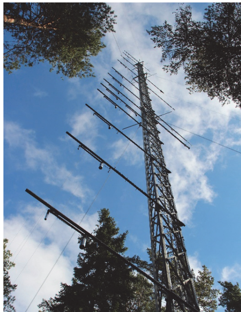
Figure 4. The 102 m tall flux tower at the ICOS Sweden Norunda station ( http://www.icos-sweden.se/station_norunda.html ). Photo by Irene Lehner.
