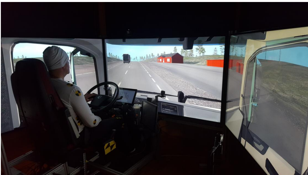
Figure 1. The simulator set up consisted of three TV-screens together with a partly physical and partly virtual truck environment.
