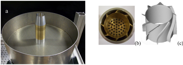
Fig. 1. (a) The burner mounted in the co-flow arrangement. (b, c) The swirl arrangement. In the center of the swirler (axial type swirler) a perforated plate bypasses a fraction of the mixture without imparting swirl.
