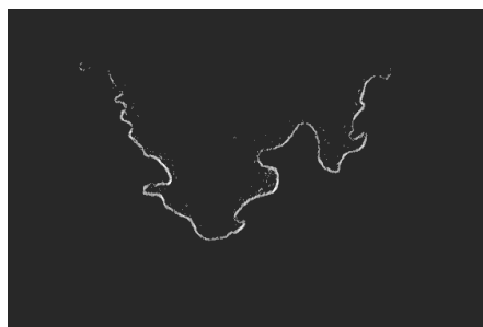
Figure 6. The maximum gradient of the OH-signal, giving an approximate representation of the flame front location for the flame in Fig. 3.
