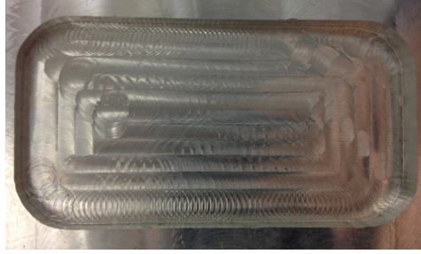
Figure 2.2 Milling task where a rectangular area of material, a so called pocket, is to be removed.
