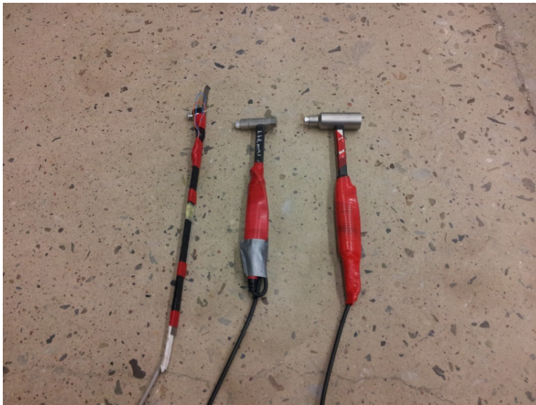
Figure 5.4: Impact hammers, from left: home-made impactor (screw/bolt) with piezoelectric crystal, hammer PCB model 086C03, hammer PCB model 086D05.
