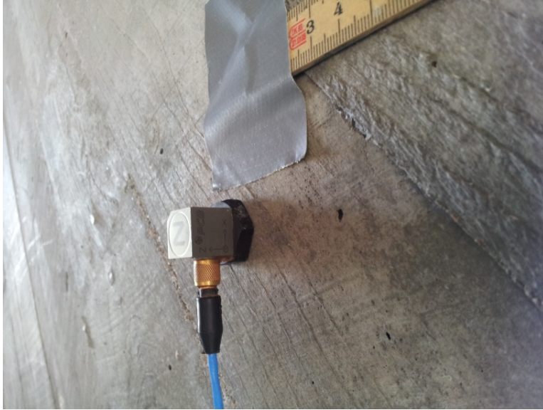
Figure 5.3: Three component accelerometer (PCB model 339A30).
