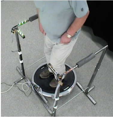
Figure 1. Stroke survivor using ActivBOSU, leaning slightly towards the right. Therefore the front-right and back-right indicators are lighted green.
