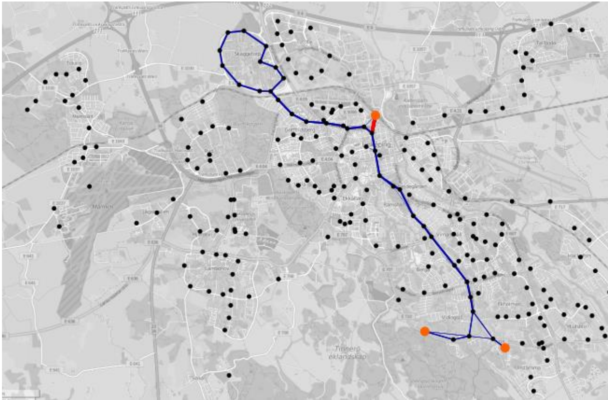
Figure 6 A map of bus line 1. Red lines show electric roads. Orange dots show charging stations. Black dots show bus stops.
