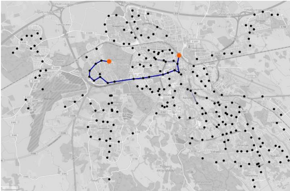
Figure 8 A map of bus line 3. Red lines show electric roads. Orange dots show charging stations. Black dots show bus stops.
