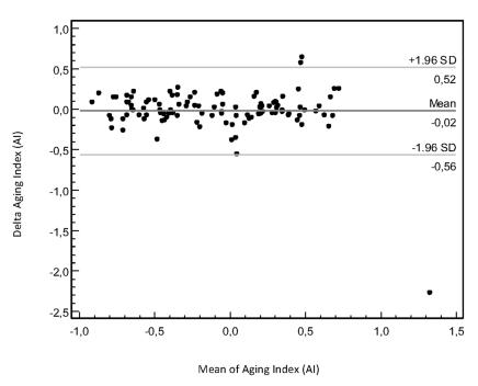
Fig 2. Repeatability of aging index. Bland-Altman plot of two consecutive measurements of aging index (AI) by the Meridian DPA apparatus, depicting the relationship of difference of measurements (Delta AI) and mean value of measurements.
