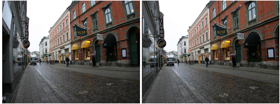
Figure 1: Left: An image taken with a fisheye lens. Right: The same image rectified when kernel voting is used to determine the radial distortion
