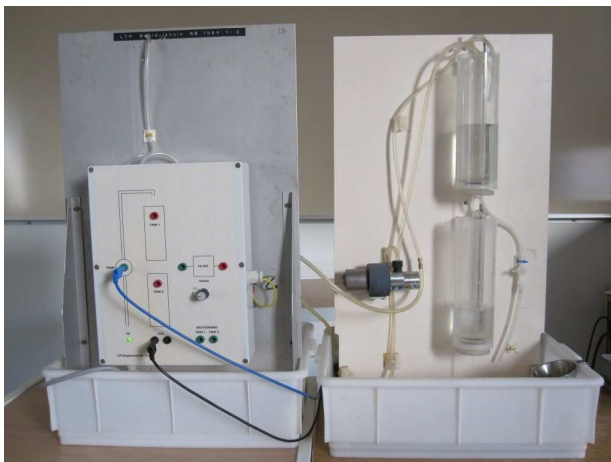
Figure 18.1 System setup. The level of the upper tank on the right is controlled through a pump. The system on the left is used to introduce a load disturbance.
