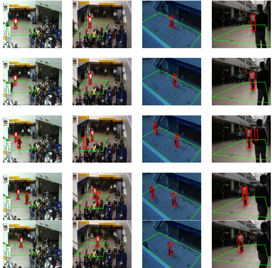
Figure 4.16: Resulting output of the tracker from frames 700-900 of scenario S1. The red boxes indicates the detected and tracked objects in the four cameras. The green rectangle indicates the area within which objects are tracked. See also pets.avi at http://www.maths.lth.se/~ardo/thesis/ .
