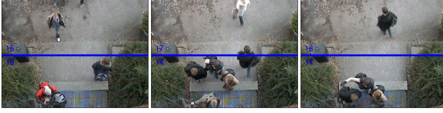
Figure 4.8: People entering and exiting an entrance. The numbers above and below the line gives the number of people crossing the line going out and in respectively. The system detects 4 people entering and 3 people exiting during the time shown in the figure, which is correct. See lunchcut.avi at http://www.maths.lth.se/~ardo/thesis/for the video.
