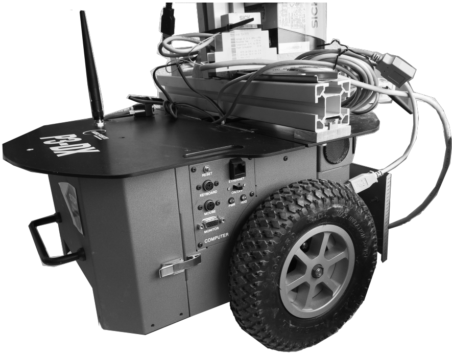
Figure 7.13 The Pioneer 3 robot used for the experiments in Section 7.6, see [MobileRobots, 2006] for more information.
