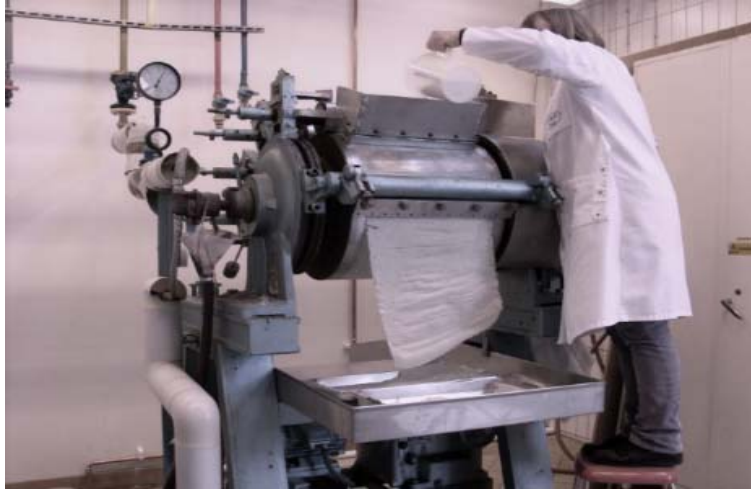
Figure 10. The drum-dryer used in the present work (Goudsche Machinefabriek) and the sheets of SMP. The average surface temperature of the drum was 115°C, and the drying duration was 40 s.
