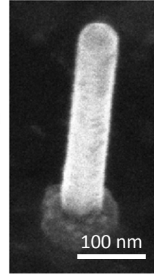
Fig 3. SEM image (30° tilt angle) of a single NW after the gate length definition.
