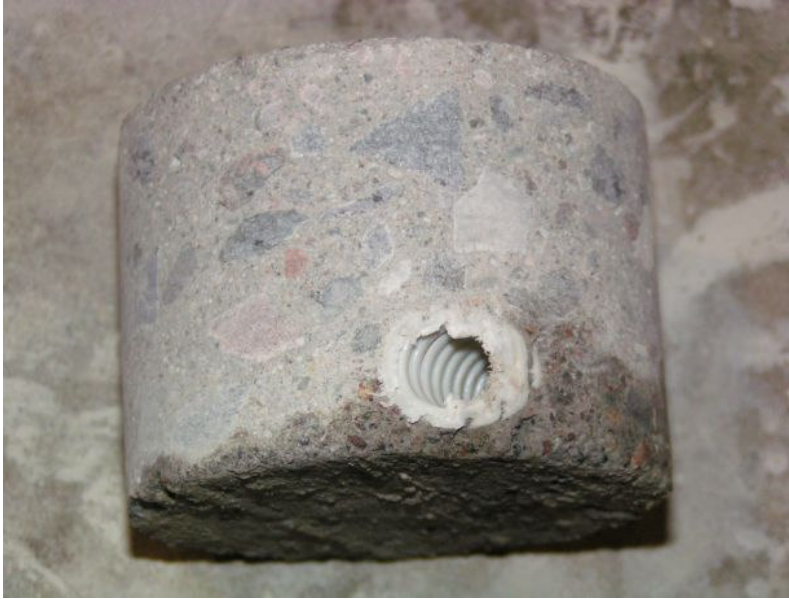
Figure 5.11 Fracture of cylinders when bond testing occurred totally within the interface between the HD/F element and the cast top layer. Note the proper filling beneath the installation tube though.
