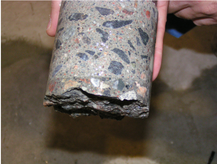
Figure 5.14 For some cores, the fracture when pull-out testing occurred in the HD/F element (the darker part at the bottom of the cylinder), which indicates on proper bond between the SCC top layer and the HD/F element.
