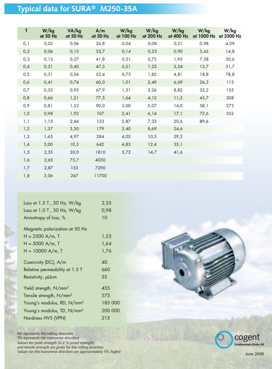
Figure D.1: Data sheet for the laminated steel plates used in the iron core, source 'Surahammar'
