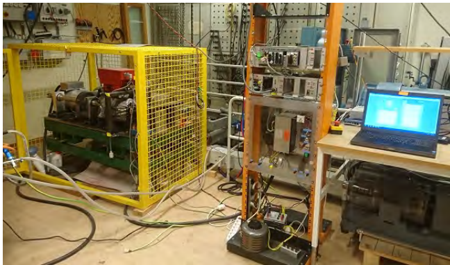
Figure A.1: The experimental setup with the parallel drive bench , the control unit and the PC
