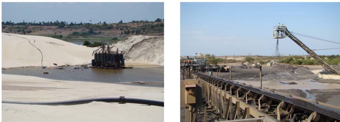
Figure 1.- Left: hydraulic separation plant of heavy minerals from coastal sand dunes at Angoche; Right: arrival of heavy minerals' wet concentrate at the magnetic separation plant in Moma coastal area.
