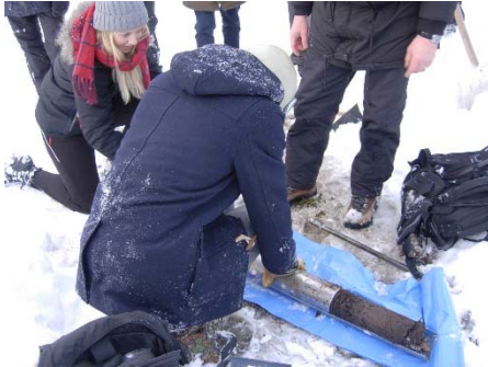
Figure 2. The core is being revealed.
