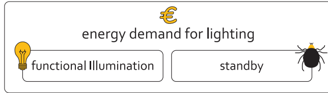
Figure 3.3 Energy demand for lighting is the sum of energy for functional illumination and energy for standby
