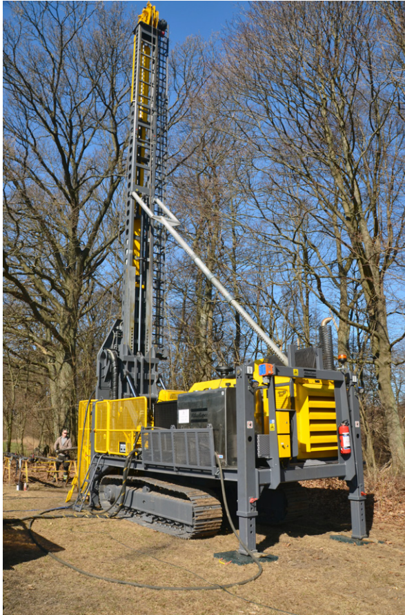
Fig. 29. The recent drilling close to the GSSP was performed by the Engineering Geology group of the Department of Measurement Technology and Industrial Electrical Engineering, Lund University, with the new Atlas Copco CT20 drill rig that will be used for the Swedish Deep Drilling Programme (SDDP). Photo: O. Lehnert.
