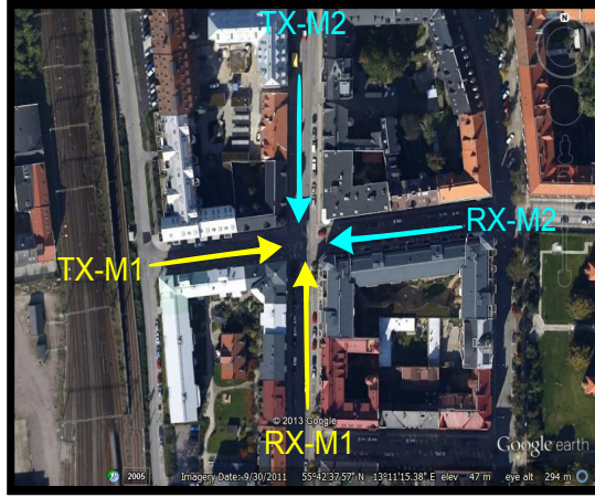
Figure 1: Google Earth TM [10] aerial image of the investigated urban crossroads scenario in the city of Lund with two vehicles moving towards the intersection at a speed of approximately 10 m/s (N55° 42' 37", E13° 11' 15").
