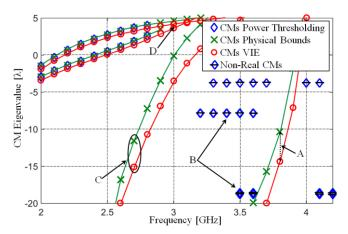
Fig. 7. Comparison of notable and interesting characteristic modes for the SIE and VIE solutions of Cube M3. Far-field CM tracking [34] was utilized to link modes at different frequencies (solid lines added) to help identify the corresponding modes for the different solutions. Non-real modes are only found in the power thresholding solution and are indicated by a black line through a blue diamond marker.
