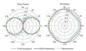
Fig. 14. Normalized simulated and measured patterns of Cube L0 for mode 2 (Magnetic CE) at 3.92 GHz. The Theta and Phi patterns are aligned with the coordinate system shown in Fig. 8 and Fig. 9.
