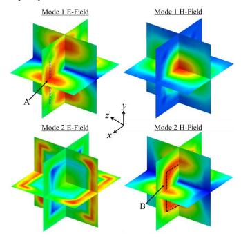
Fig. 8. *xy*, *xz*, and *yz* cross sectional cuts of the electric and magnetic nearfields (magnitudes only) for modes 1 and 2 of Cube L1. The dashed line in region A corresponds to a predicted location to place an electric coupling element which will couple electric energy into mode 1, whereas the dashed line in region B corresponds to a predicted location of a magnetic coupling element which will feed couple magnetic energy into mode 2.
