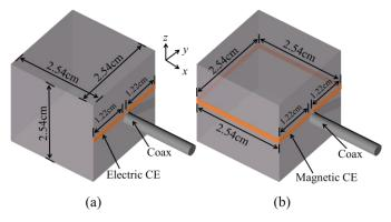
Fig. 9. (a) The electric CE and (b) the magnetic CE were designed using the CM cross-sectional near-fields. The loaded resonance frequency of both CE structures are not resonant near the characteristic modal resonance frequency.
