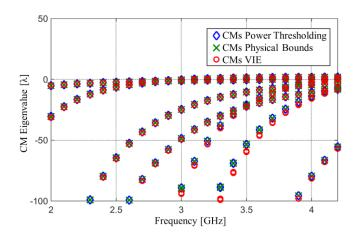
Fig. 4. Comparison and visualization of the all the SIE and VIE CM solutions between  $-100 < \lambda < 50$  for the loss free cube (Cube NL).
