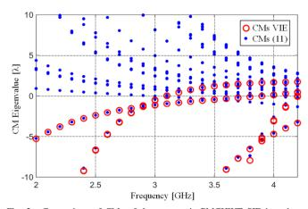
Fig. 3. Comparison of CMs of the symmetric PMCHWT SIE impedance matrix (11) and the CMs of the VIE formulation for Cube L0. The symmetric SIE impedance matrix produces several inductive modes near resonance, these are non-real modes as this structure does not support inductive eigenmodes at frequencies below 3GHz.
