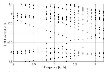
Fig. 2. First 25 CMs of the non-symmetric PMCHWT impedance matrix which are near resonance. In particular, 12 modes are near resonance at 2GHz, where the structure is electrically too small to support any near resonant modes at this frequency.
