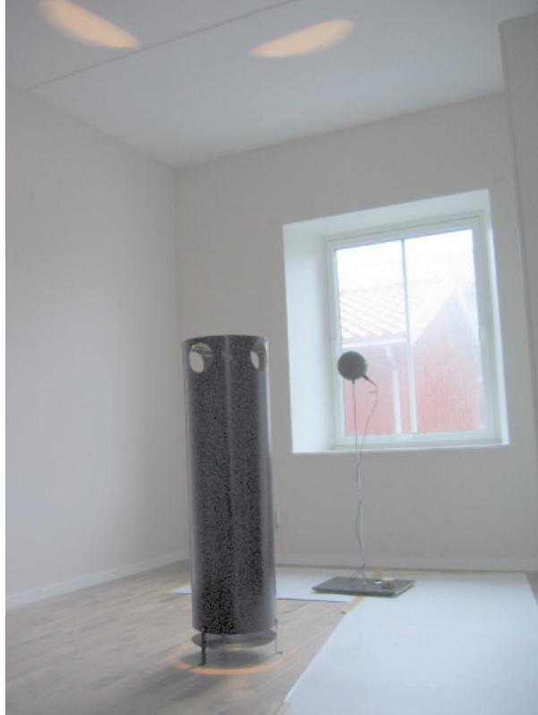
Figure 4.39 Measurement of operative temperature in one bedroom in the test apartment.
