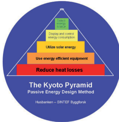
Figure 2.2 The “Kyoto pyramid” showing schematically the passive design principles (Husbanken/SINTEF Byggeforsk, Are Rødsjø/Tor Helge Dokka).
