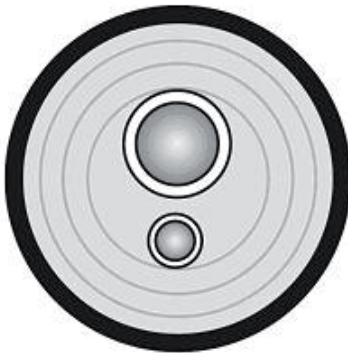
Figure 4.51 Distribution pipes for domestic hot water, placed in the ground (Picture: Uponor, 2006).
