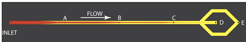
Figure 5.12. The principle behind the plasmapheresis chip. Multiple outlets are placed along the separation channel where red blood cells focused in the middle of the channel are subsequently removed. The clean plasma fraction is collected at outlet E.
