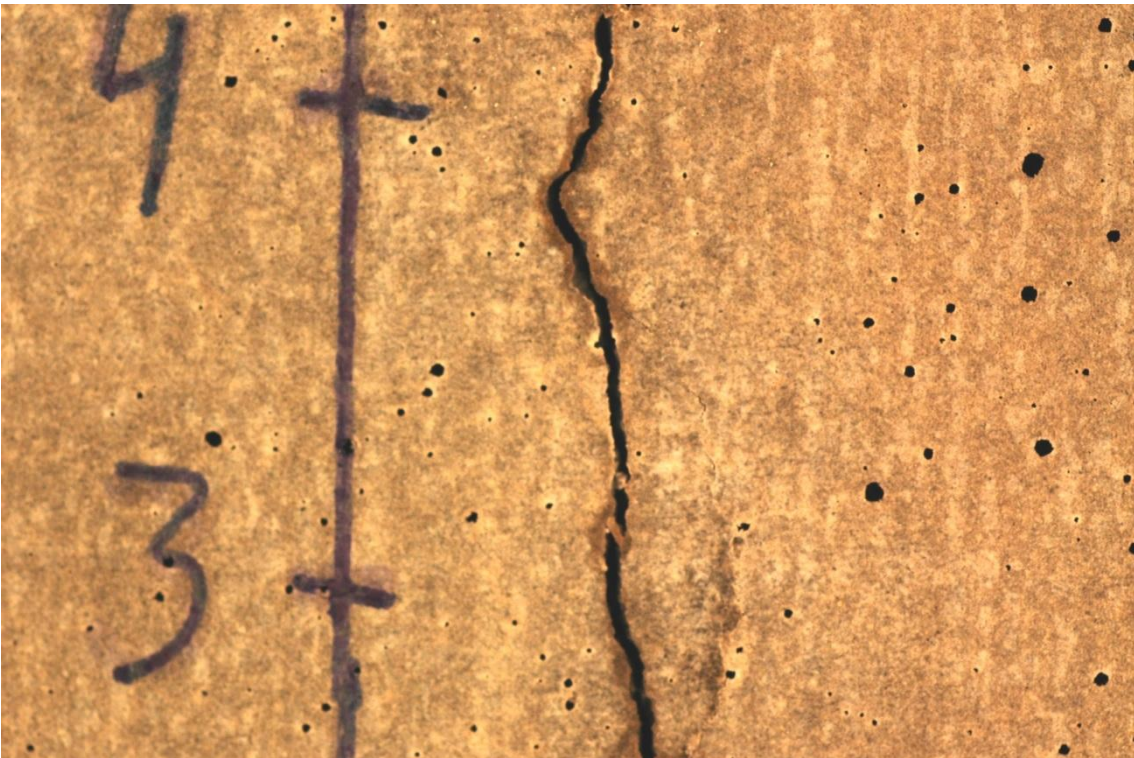
Figure A2.4: 0.4 mm crack after 1 year cyclic immersion in sea water and drying. Test series 1, specimen H75-4-2-1.
