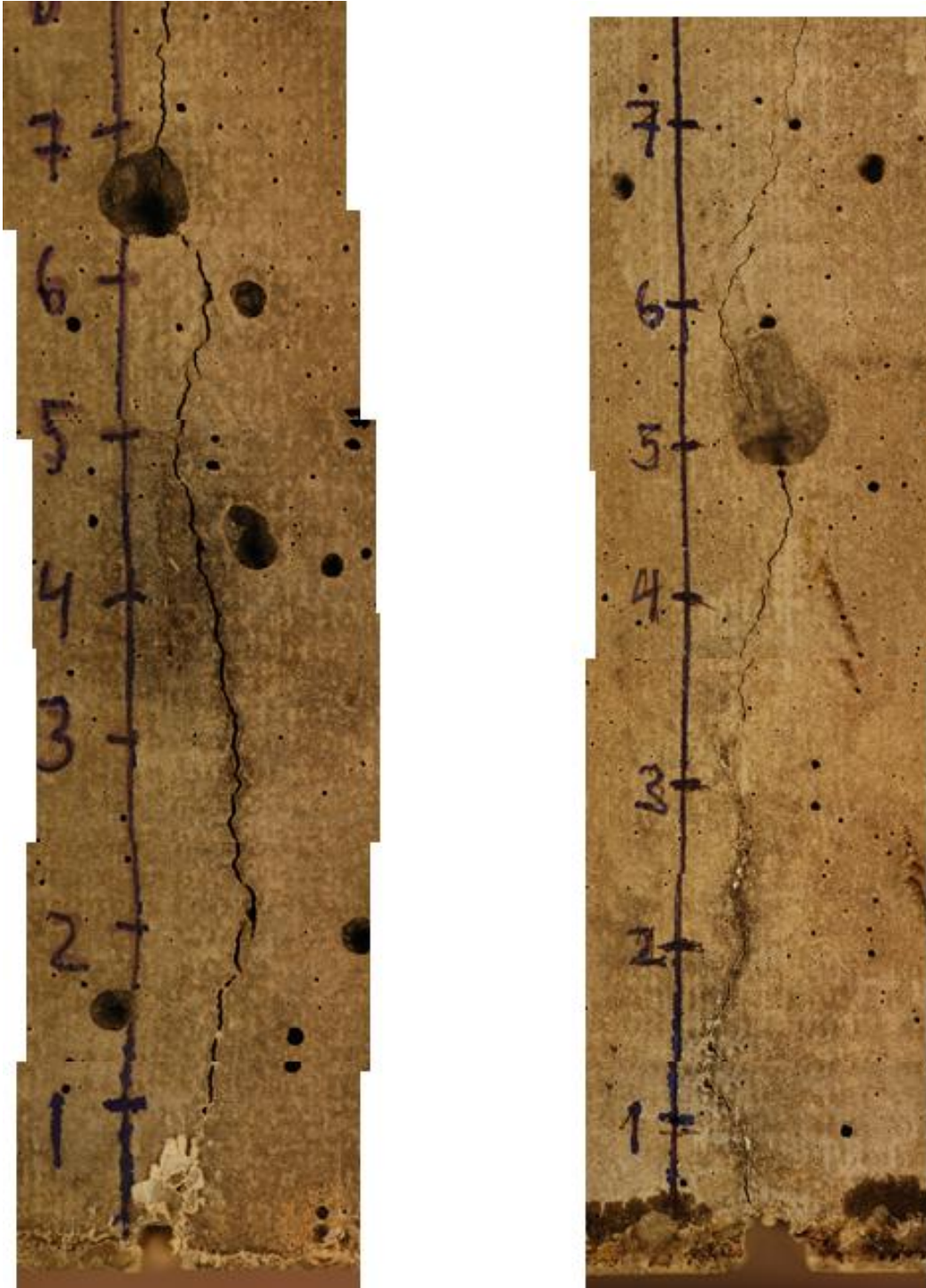
Figure 12.1: Photographs of cracks after exposure. The same specimens as in figure 7.1.
