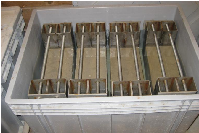
Figure 10.1: Water exposure type 1; permanently under water.
