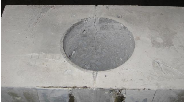
Figure 13.1: Example of a specimen after the core has been drilled out.
