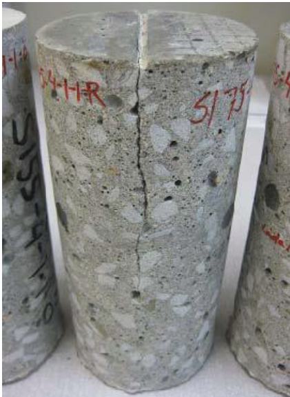
Figure 13.2: Example: core drilled out from specimen S1-75-4-1-1-R (75 mm cover, crack width 0.4 mm, permanently exposed to pure water).
