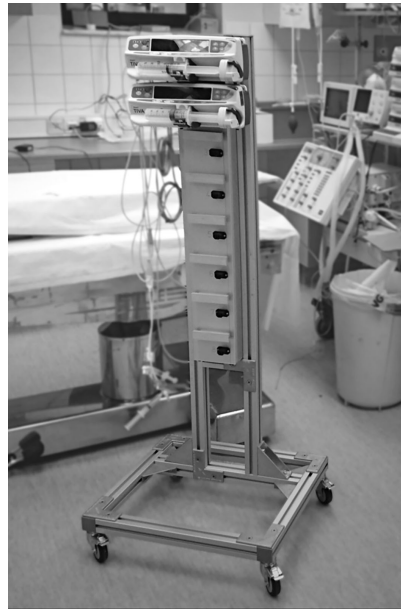
Fig. 4: Prototype closed-loop hemodynamic stabilization system, with two (out of eight possible) computer controlled infusion pumps attached. Connectors for blood pressure transducers and user interface PC are situated on the backside of the column.
