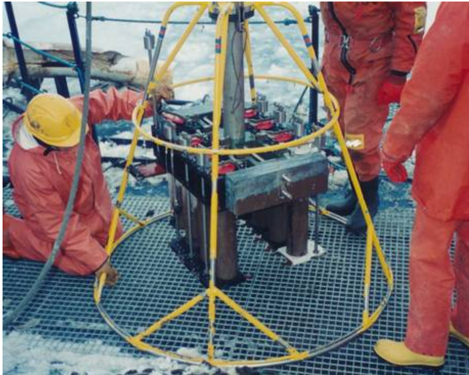
Figure 6-15 The sediment core sampler
